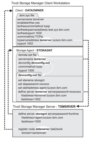
Figure 9. Communications information. Results of Steps 2.1 and 2.2. The passwords are shown as "xxxxxxx" because they are encrypted in the file.
